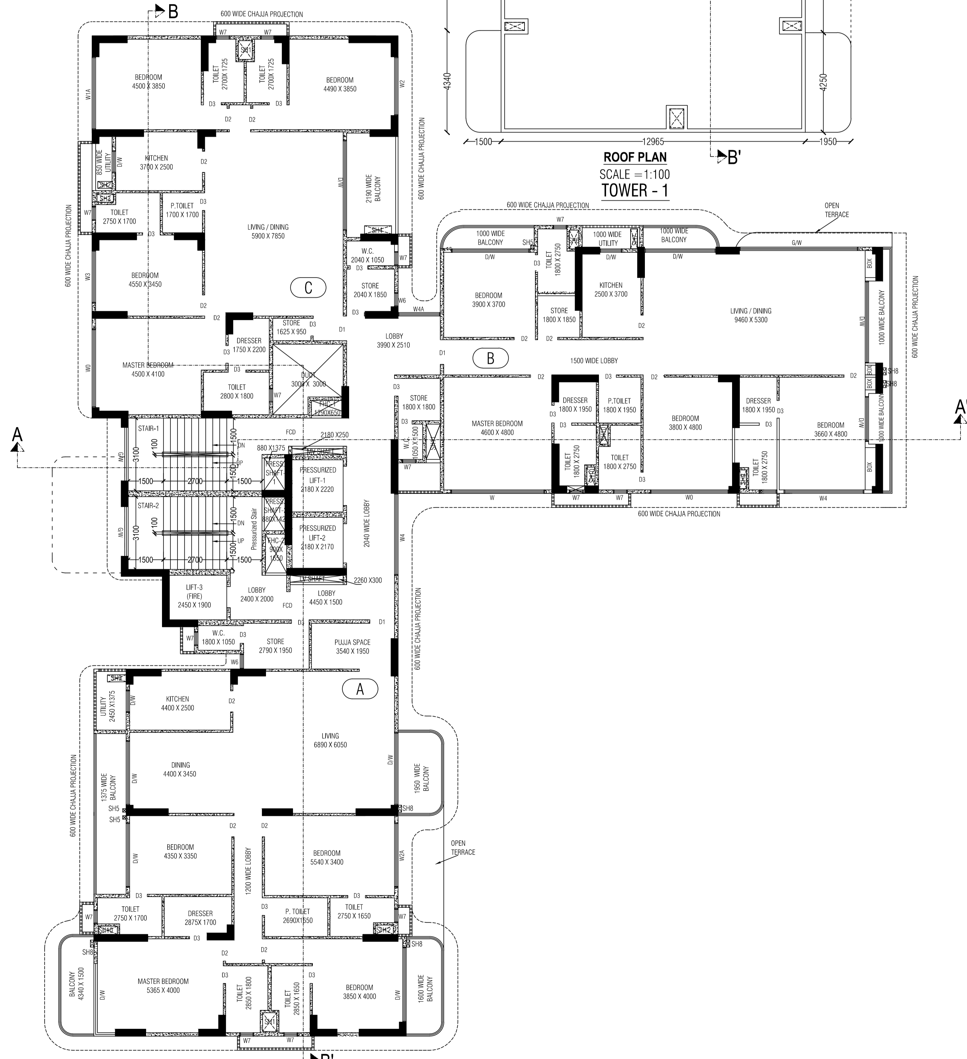
4TH, 6TH, 8TH, 10TH, 12TH, 14TH, 16TH, 18TH, 20TH, FLOOR PLAN SCALE = 1:100 BLOCK-A TOWER - 1
