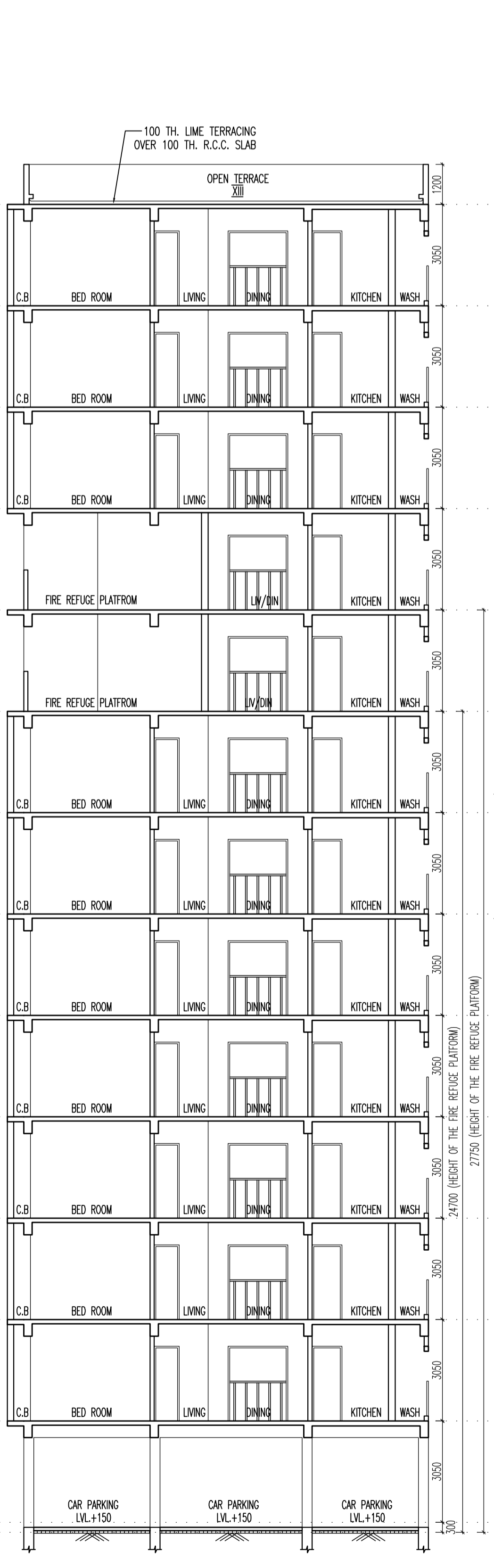
SECTION AT C-C TOWER - 2 SCALE=1:100
