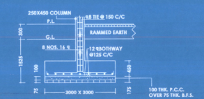
DETAIL OF 250X450 R.C.C. COLUMN FOUNDATION SCALE - 1:100
