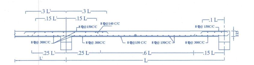
TYPICAL DETAILS OF R.C.C. ROOF SLAB (S)
