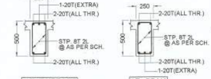
DETAILS OF BEAM MKD. B2(250x500) SCALE 1:30
