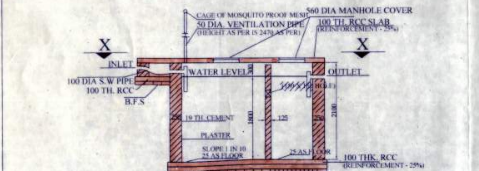
SECTION OF SEPTIC TANK
