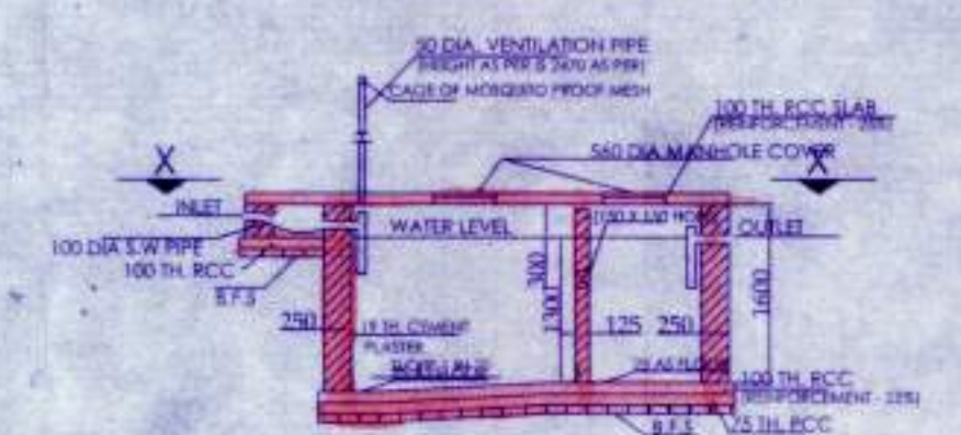
SECTION OF SEPTIC TANK
