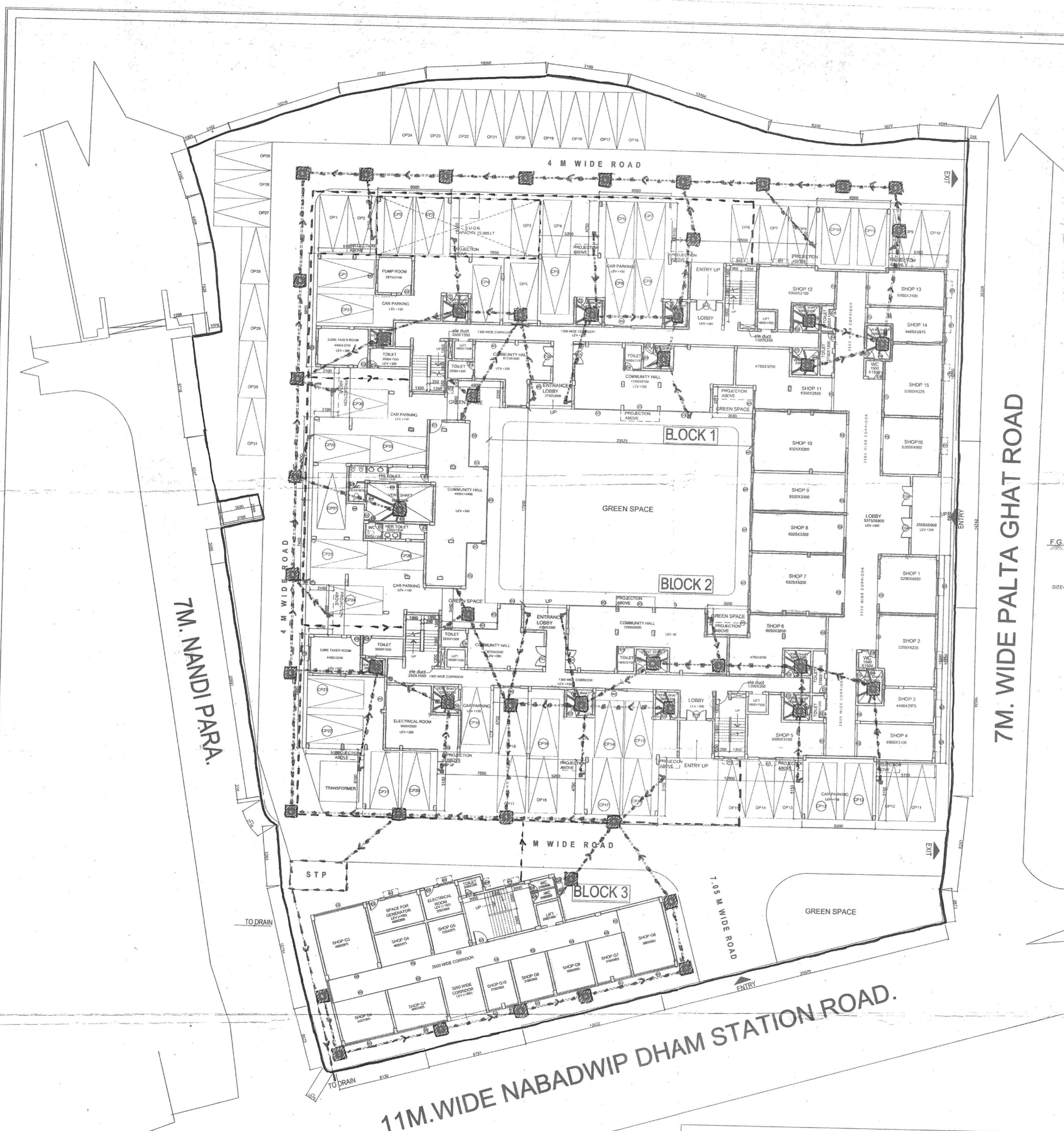
OVER ALL SITE PLAN SHOWING GROUND FLOOR PLAN AND SEWER LINE CONNECTION LAYOUT SCALE 1:150
